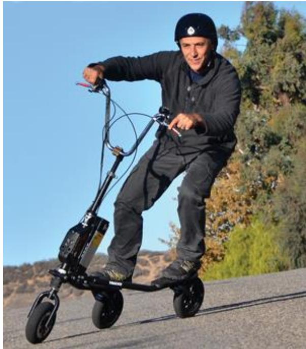
Gildo Beleski, chief technical officer and designer for Trikke Tech, rides the Trikke Freedom on a Buellton street. This Trikke has an electric motor in its front tire and a lithium battery, seen just in front of his right ankle, but you can operate it with the power off.
