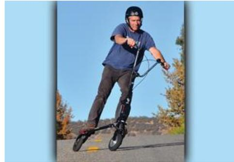
Gildo Beleski, chief technical officer and designer for Trikke Tech, rides the Trikke Freedom on a Buellton street. This Trikke has an electric motor in its front tire and a lithium battery, seen just in front of his right ankle, but you can operate it with the power off.
